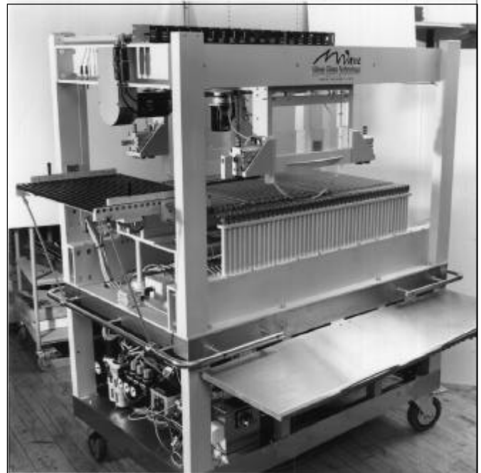
The finished model of the glass-plate processing machine.
